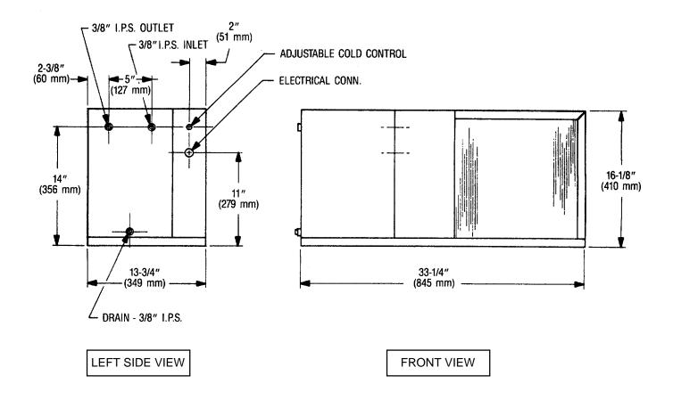
NOTE: This unit is intended for remote installation only. It is important to insure proper ventilation. Allow a minimum clearance of 18 inches in front and 18 inches in the rear of unit.
